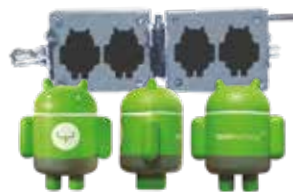
STEP 2 A PLASTER & ALUMINIUM MOULD IS PRODUCED FOR PRODUCTION
